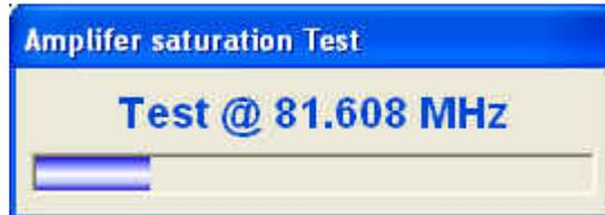
The test verifies the difference specified in EMC regulations between the power calculated during the calibration phase with the limit 1.8 times that of the test ( $P_c$ ) and the power to be applied during the testing phase ( $P_t$ ). If the outcome is positive, the amplifier is not saturated and the system is suitable for the immunity test.
