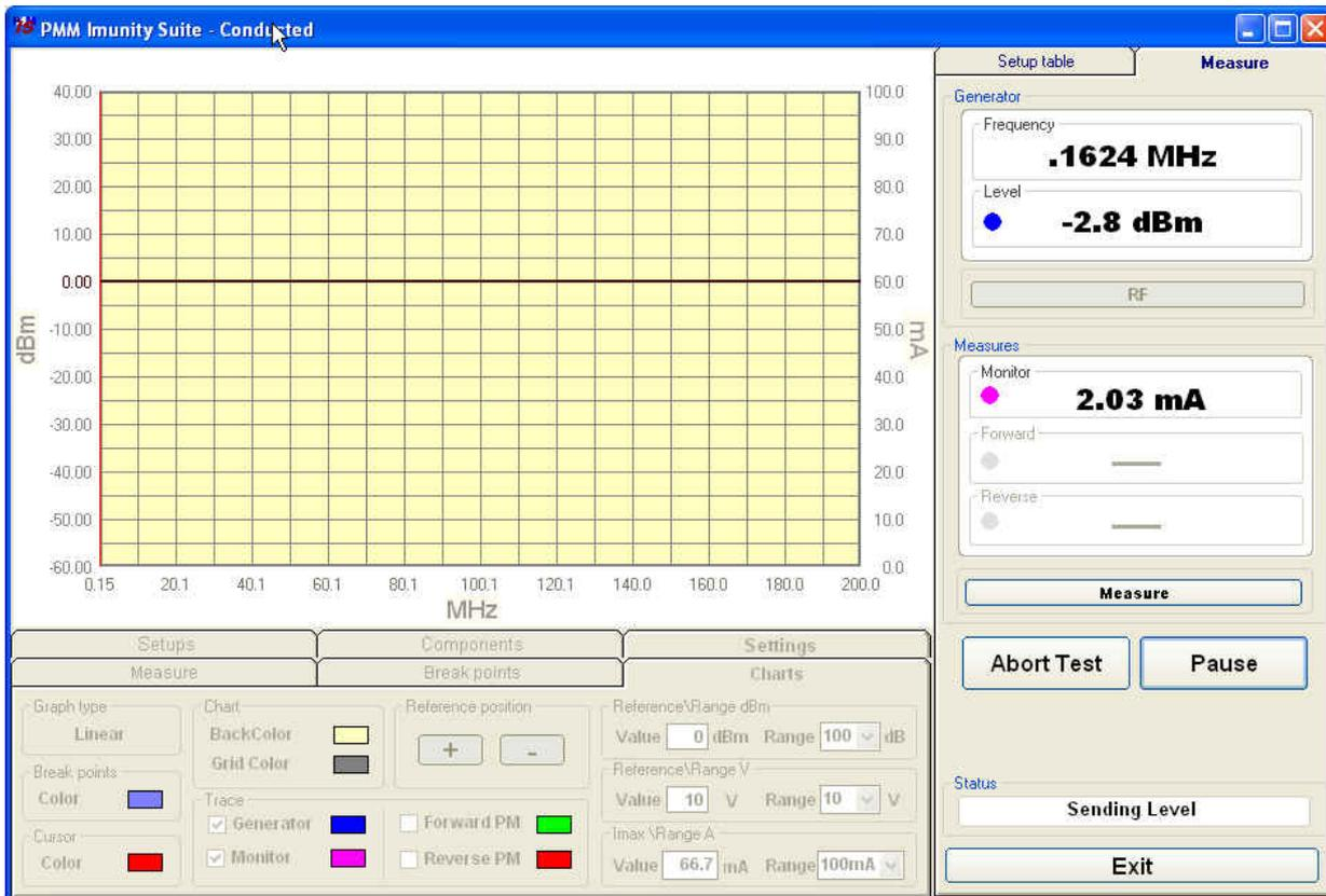
The example below shows the current and the generator level during a test in which the current limit is exceeded and then brought back into range by the software. The correct generator levels will be saved and used during the second sweep.
