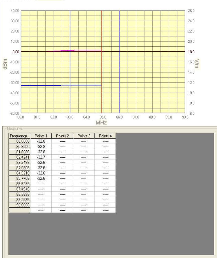
Because the immunity test is only valid if there is an area within the shielded chamber where field uniformity complies with the standard, the field sensor has to be arranged in different positions. The program keeps track of those positions in the following window:
