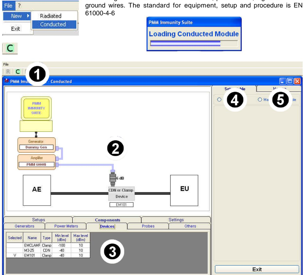
Fig. 4-1 Main window - Conducted
