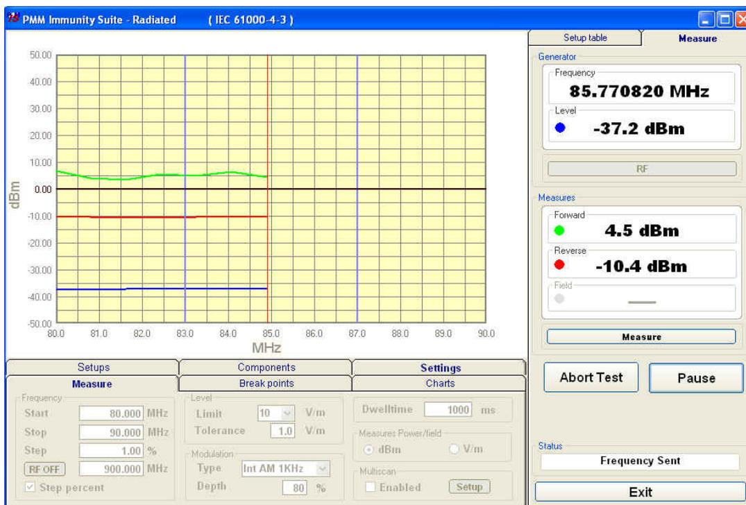
During the test, the **Generator** window shows the level extrapolated from the setup table and used by the generator to obtain a constant magnetic field in the selected frequency range. The color of the dot corresponds to the color of the line on the graph.
