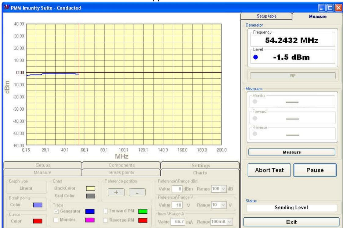
During the test, the **Generator** window shows the level extrapolated from the setup table and used by the generator to obtain the required voltage.
