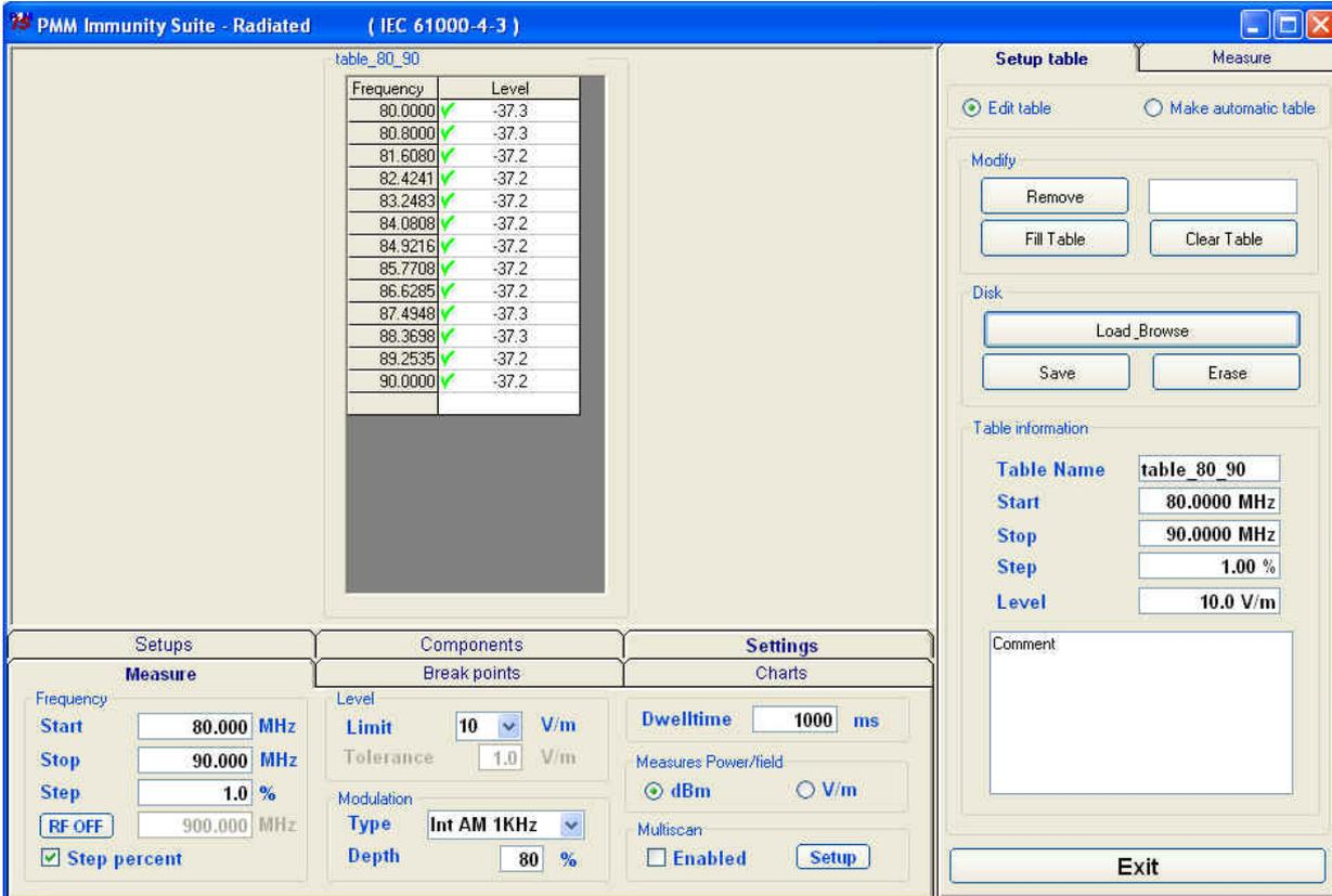
The screenshot shows the 'PMM Immunity Suite - Radiated ( IEC 61000-4-3 )' software interface. The main window displays a table named 'table\_80\_90' with the following data:
