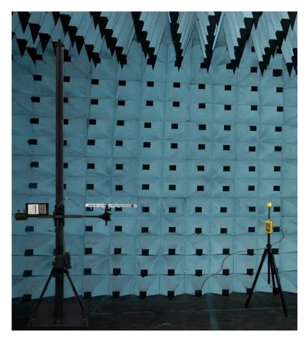
The possibility of storing the different lists of frequencies in the internal memory of the PIRS during the field calibration, as well as the possibility of having the power signal at the "N"connector output allows the operator to take advantage of all the power generated and directly available to the transmitting antenna connector, without attenuations due to the coaxial cable which sometimes can even exceed 6 meters in length (height 4 meters of mast + section to reach the amplifier room)
