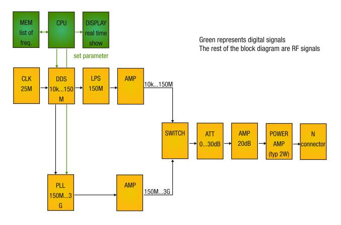
The system receives as input (through its software) a list of frequencies that the CPU (Central Processing Unit) transmits to the DDS (Direct Digital Synthesis).
