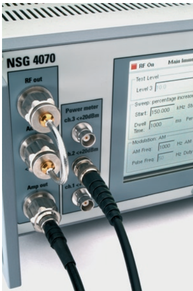
NSG 4070 front panel with RF ports
