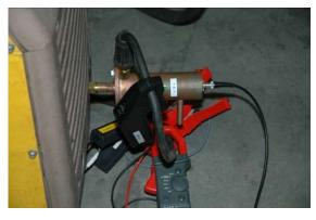
Welding machine with shunt and current clamps
