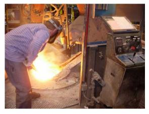
Operator working at open metal induction heater
