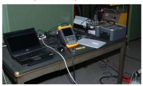
Scopes for measuring the voltage- current waveform
