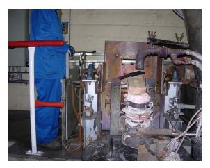
Operator working at a small closed gold melting oven
