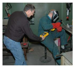
B-field measurement on the welder's body
