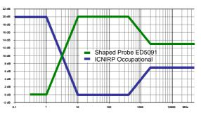
Principle of the Shaped Probe: Automatic evaluation in a given frequency range. The probe sensitivity corresponds to the inverse of the limit value curve. The test equipment shows the result as "% of STD" i.e. as a percentage of the limit value of the chosen standard (ICNIRP Occupational in this case).
