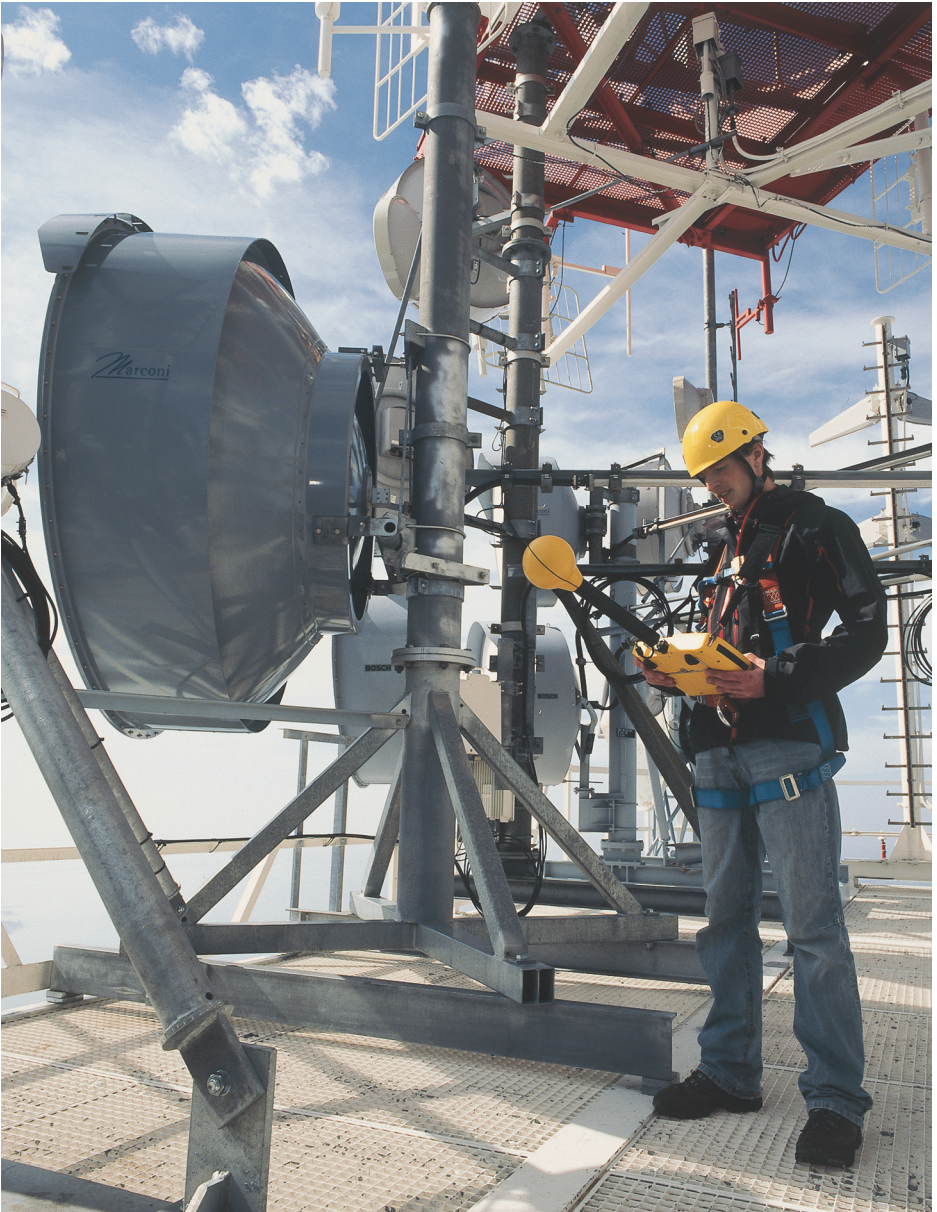
Figure 1: SRM-3006 in on-site use
