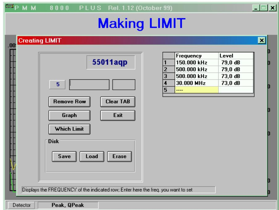
To assign frequency and level values just click on the desired row with the mouse and directly type in the frequency value and the level in dB.
