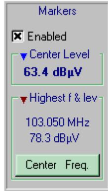
The **Center Level** marker is shown in the spectrum window by a small blue arrow and the read level value is displayed.
