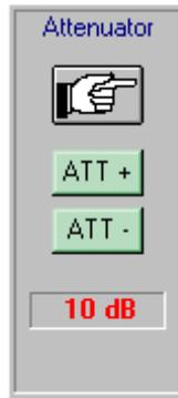
The manual attenuator can be inserted or excluded using the
