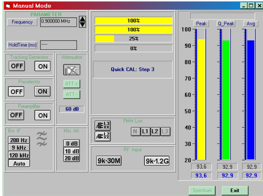
During the autocalibration four increasing bar will show the calibration progress. As soon as all steps are done, PMM 8000 Plus exits the calibration window and the calibration is finished and saved.
