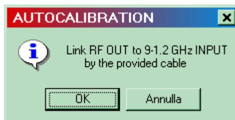
Either Quick CAL or Full CAL can be performed, normally only Quick CAL is required for level correction, with Full CAL the preselector filters centering is also performed.
