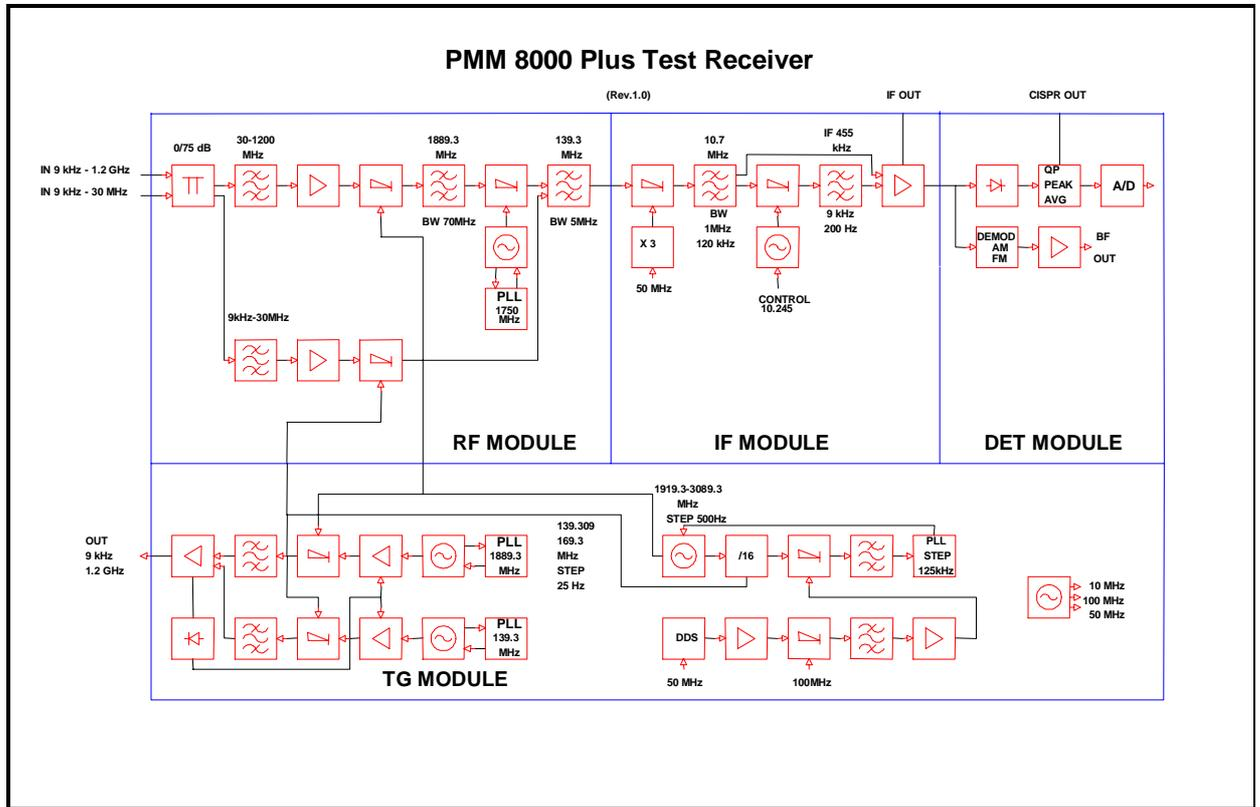
Fig. 1-3 PMM 8000 Plus Functional Diagram
