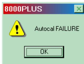
If the case try first to change the calibration cable provided, otherwise the equipment need to be repaired, contact your PMM representative.
