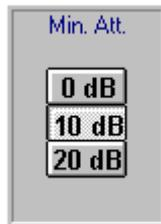
This window allows the minimum attenuation to be set either to 0, 10 or 20 dB. When the minimum attenuation is active, the manual attenuator cannot be lowered under the set value. The value set is showed in lighter gray color.
