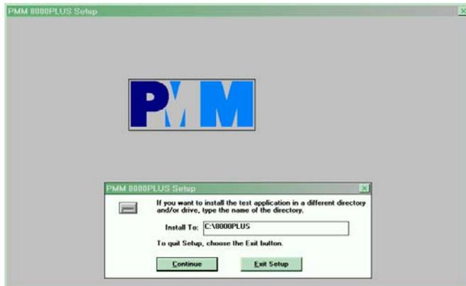
Click on the **Continue** button to continue with the installation procedure, or **Exit Setup** to abort it. Near the end of the installation procedure the program will ask if the demonstration program is to be also installed.
