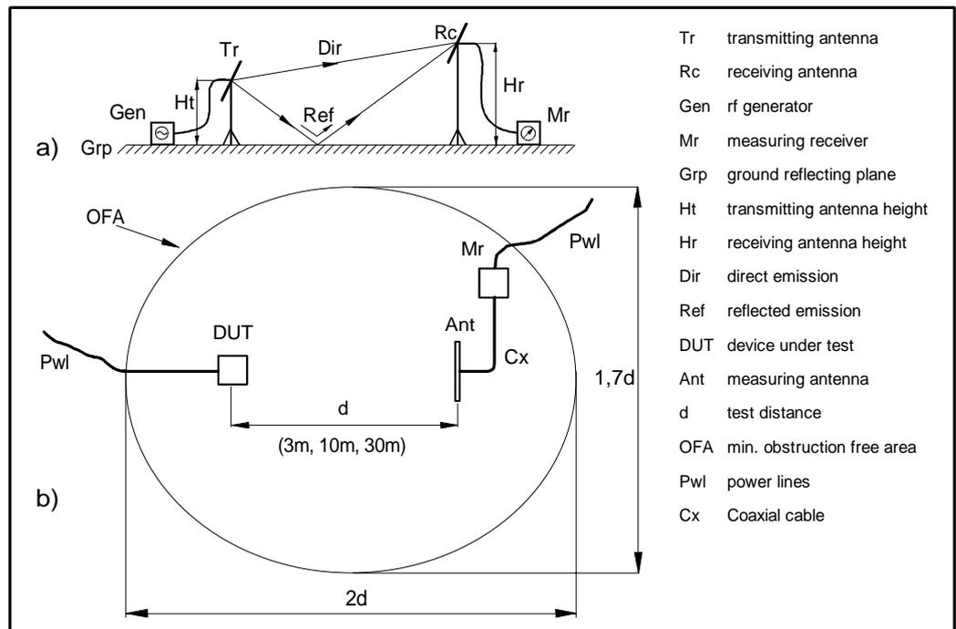
Fig. 7-5 RFI Field strength Principle: a) Reflecting ground; b) Test Site
