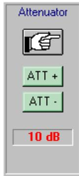
The manual attenuator can be inserted or excluded using the
