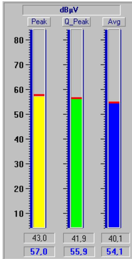
Either analog and digital readout are available in this window.
