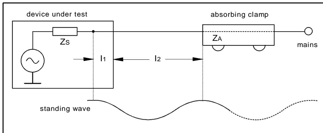
**Fig 7-3 Parameters involved with RFI Power Measurement**
