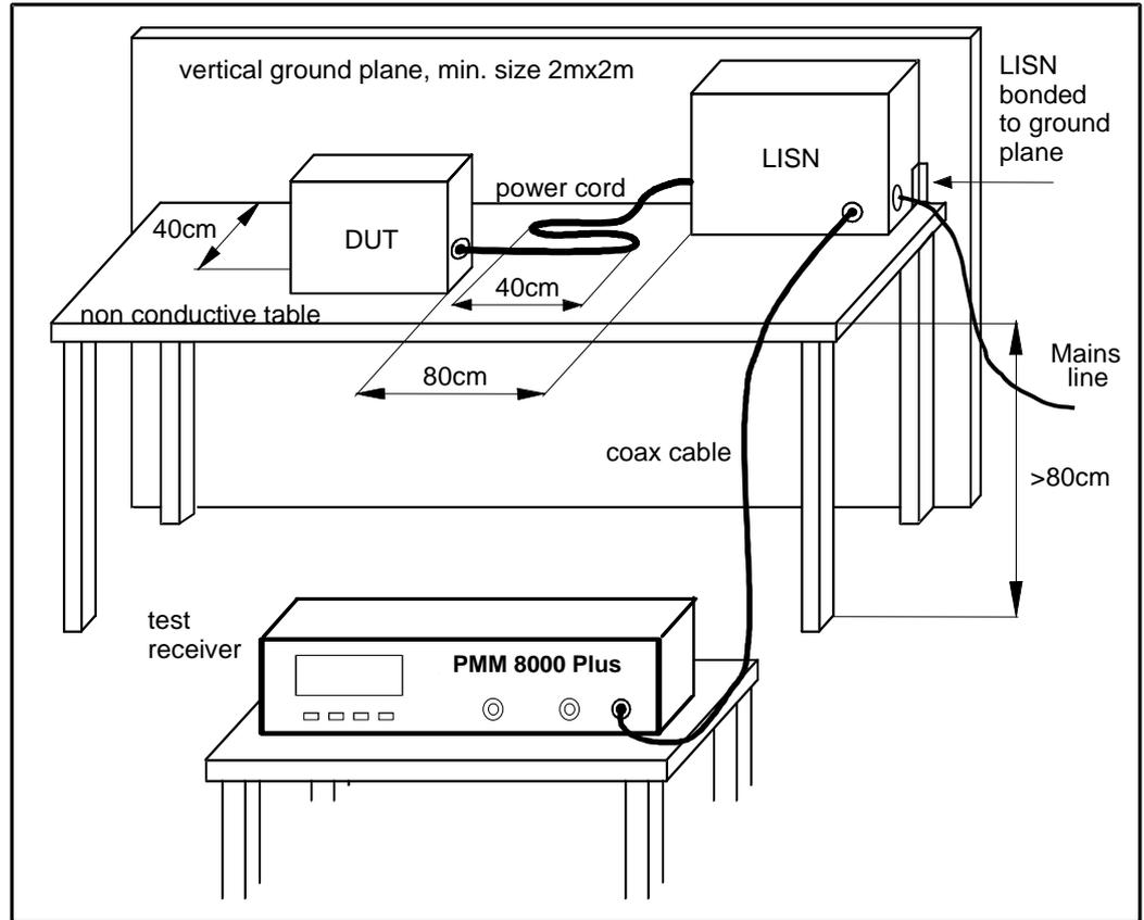
**Fig. 7-2 Example of Test Setup for RFI Voltage Measurement**
