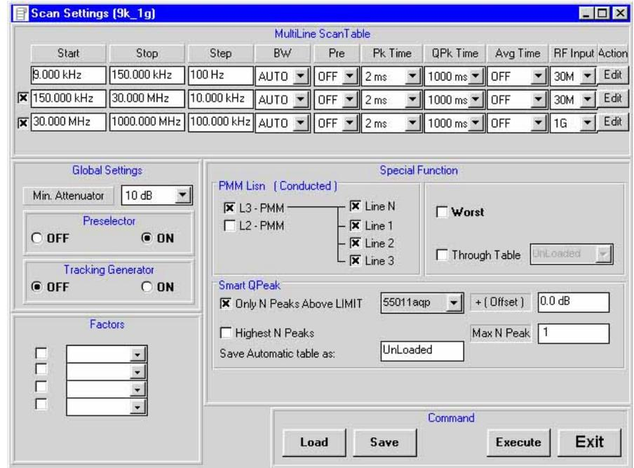
As the configuration is finished the user can either select to **Save** it into a **ScanTab** file that will store configuration data in a program proprietary format (\*.ST9) for next measurement the file can be loaded clicking on the **Load** button.
