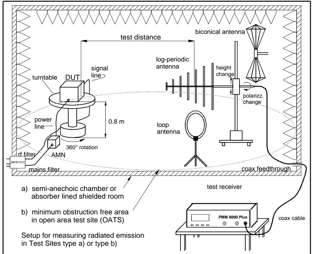
**Fig. 7-6 Test Setup for RFI Field strength Measurement**
