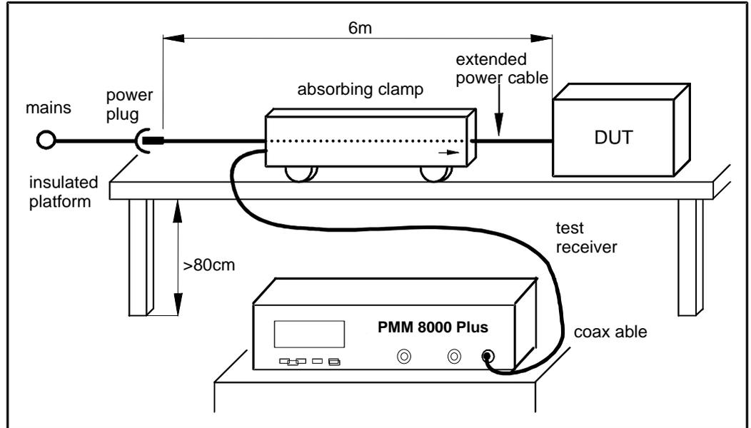
**Fig. 7-4 Test Setup for RFI Power Measurement**
