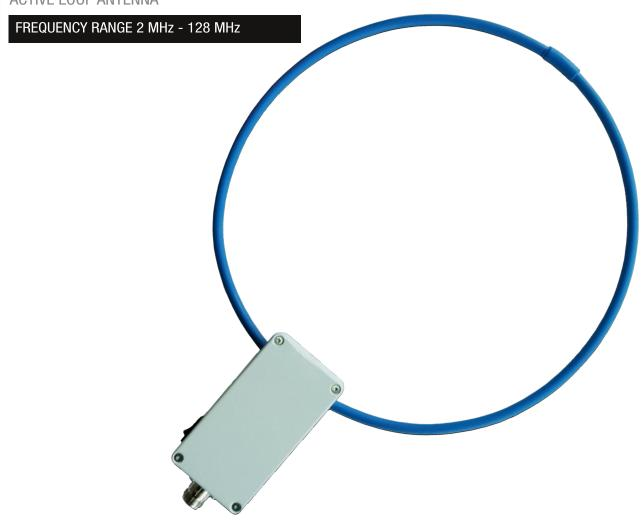
The L4-A is an active loop antenna for the magnetic component of the electromagnetic field for EMI or shielding effectiveness measures. It has a low noise preamplifier which increases overall measurement sensitivity. This antenna is powered by 4 AAA replaceable batteries (1.2 V or 1.5 V).
