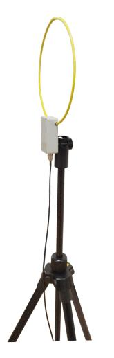
Through the 1/4" thread the L2-A active loop antenna can be easily plug on the NMR-01 amagnetic and non reflective tripod.
