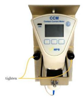
Figure 7-4. Set Up JIG
