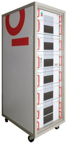
Designed specifically for radiated EMC testing, this mismatch tolerant class A amplifier delivers power continuously into the poor and variable match typically associated with testing above 1 GHz. Although antennas are usually well matched at these high frequencies, the presence of the EUT in the path of the antenna causes high levels of reflected power which only fully class A amplifiers can handle.
