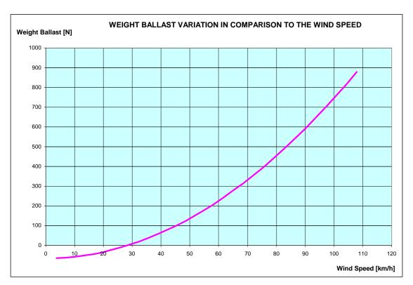
Fig. 9-3 Weight Ballast variation in comparison to the wind speed for AMB-8057/01 and AMB-8057/03 without joint
