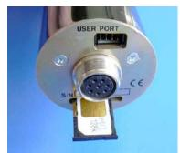
Fig. 4-3 SIM card installation
