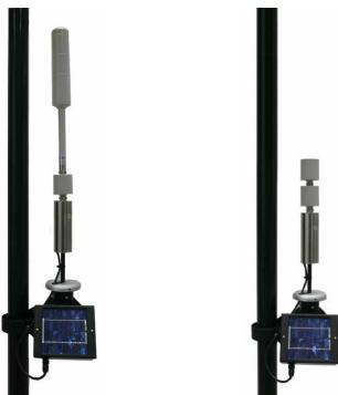
**Fig. 6-2** Dual probe configuration (internal view): EP-1B-01 mounted as secondary probe
