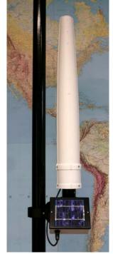
Fig. 6-4 AMB-8057 area monitor Dual-Probe configuration
