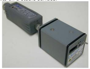
Disconnect the PMM 6630FOA from the Power Sensor holding it from the ring nut.
