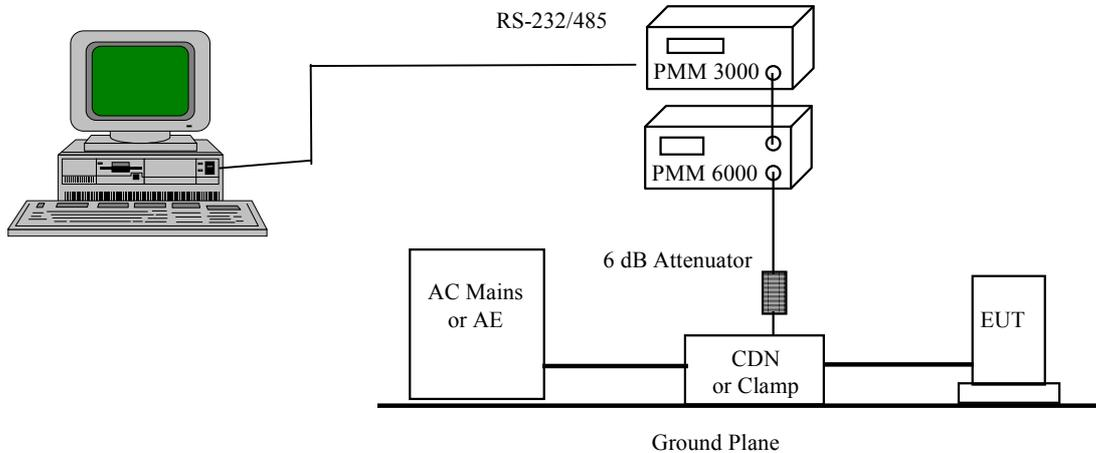
**Fig. 1-1** Connections between components
