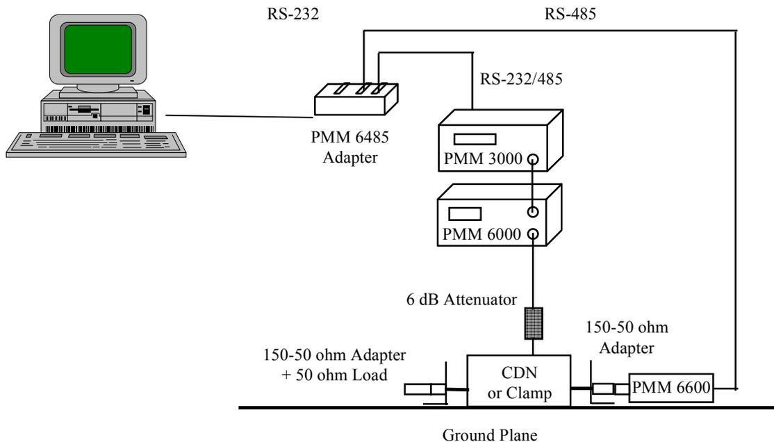
Fig. 4-1 Block Diagram of a Typical Calibration Set-Up
