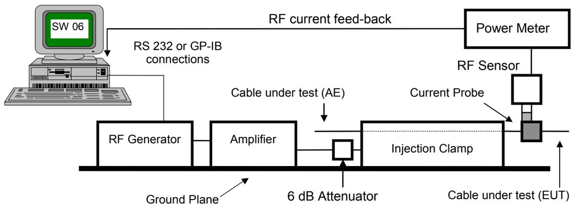
**Fig. 6-1** Block Diagram of Test Setup with Injection Clamp
