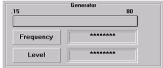
The **Generator** area indicates the generator's frequency and level output in real-time, together with test progression via an increasing horizontal Blue Bar.
