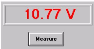
The “**Measure**” button enables a reading from the power meter. The window above the button shows, even if not pressing the Measure button, the open-circuit value of the voltage signal at the EUT connection port of CDN or Injection Clamp during the calibration phase.
