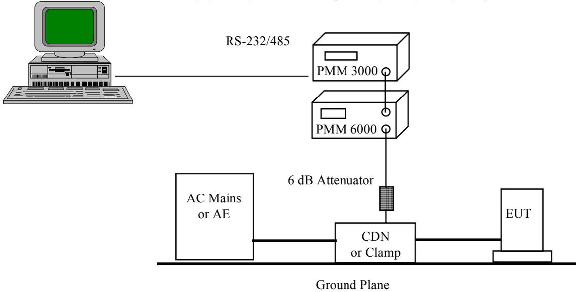
**Fig. 1-2** Block Diagram of a Typical Conducted Immunity Test Set-Up
