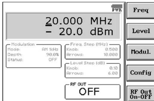
This is the operating mode in which the instrument works as a common stand alone signal generator.
