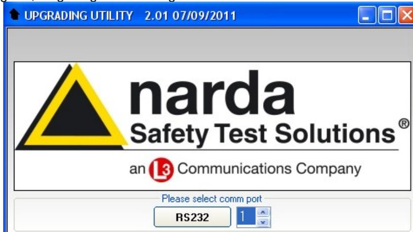
Two firmware components can be updated by this application: Firmware, which is the receiver internal program, and FPGA, to update the internal programmable logic.
