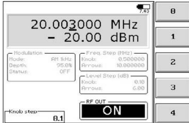
The frequency step of the rotary knob can be directly edited into this window, inputting data through the five Function Keys as usual.
