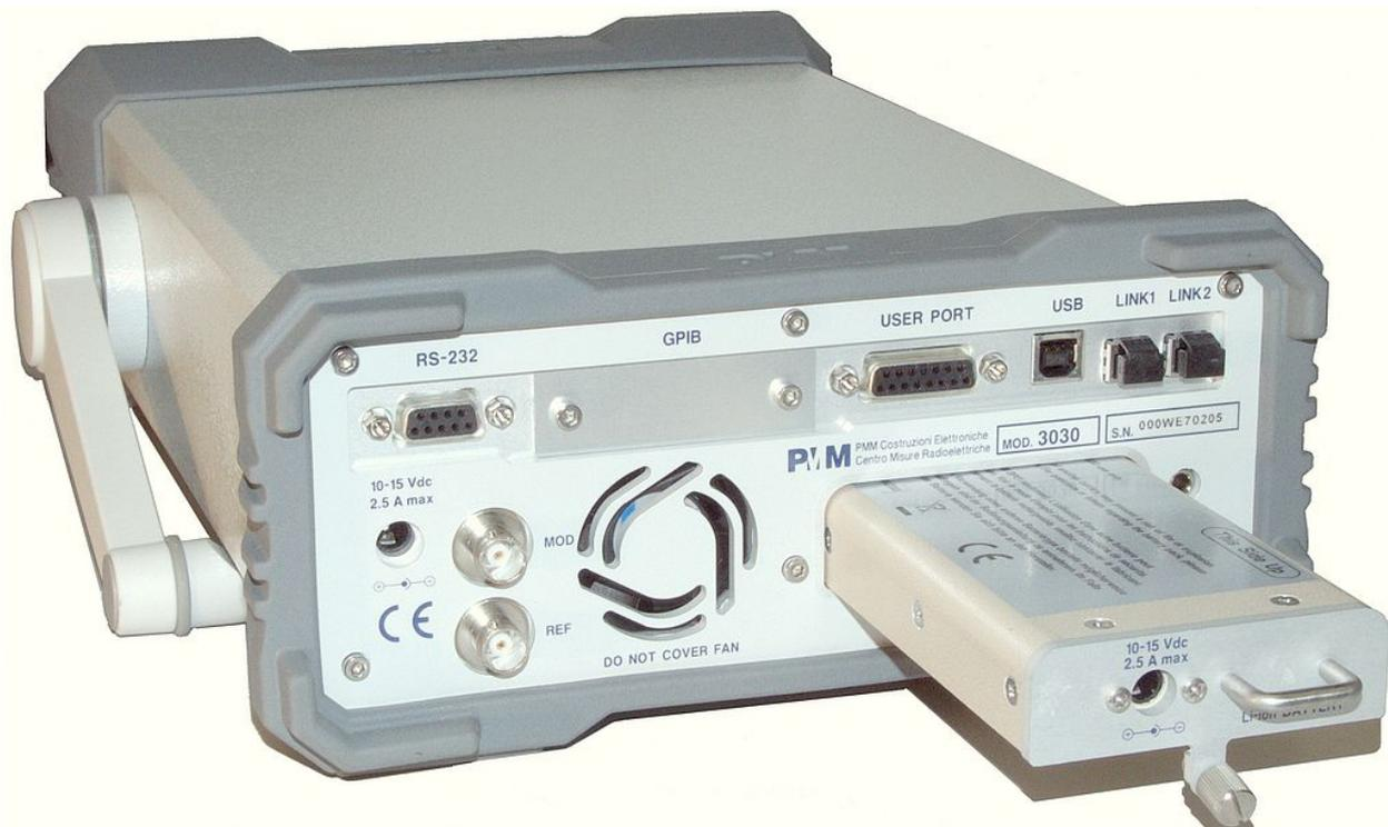
Fig. 1-5 BP-01 Replaceable Battery
