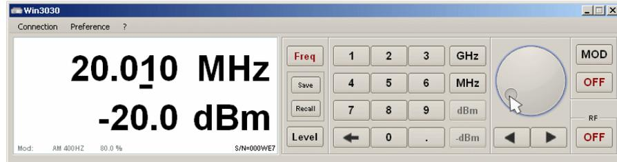
The value over the cursor can be changed by pointing and rotating the graphical knob on the screen with the mouse or using the arrow keys on the keyboard of your PC.
