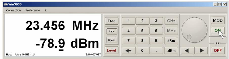
Press the button under MOD to switch ON or OFF the modulation selected.
