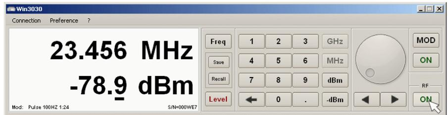
Press RF button to switch the output ON or OFF.
