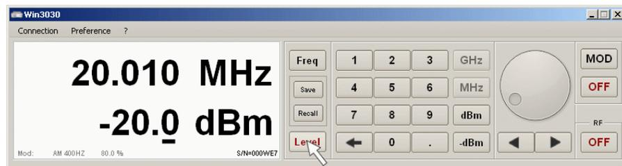
The frequency and level values can also be entered using the softkeyboard. After entering the digits, with the eventual decimal point, of the frequency value, it is necessary to press the unit among MHz and GHz. The same for the level where the unit can be dBm, for positive values and -dBm, for negative values.
