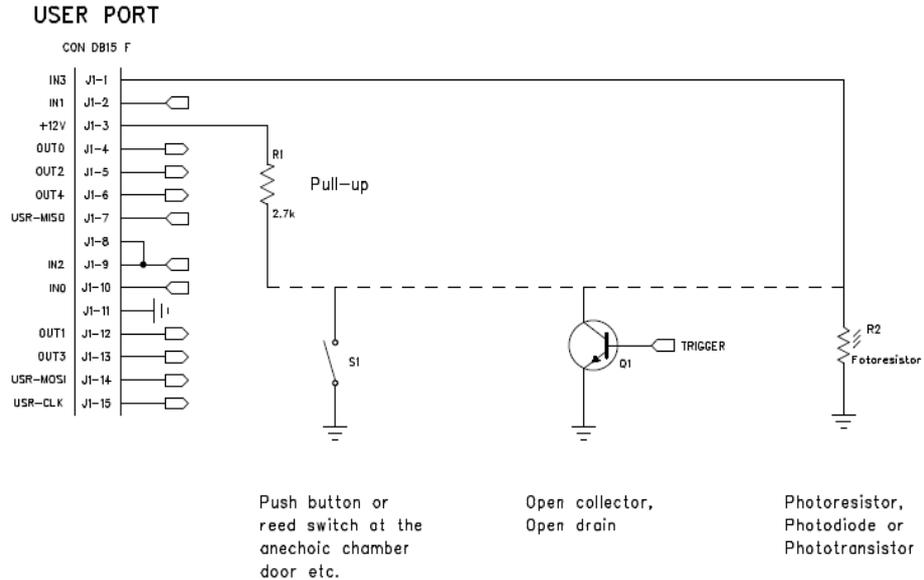
Fig. 2-2 Example of INTERLOCK circuits
