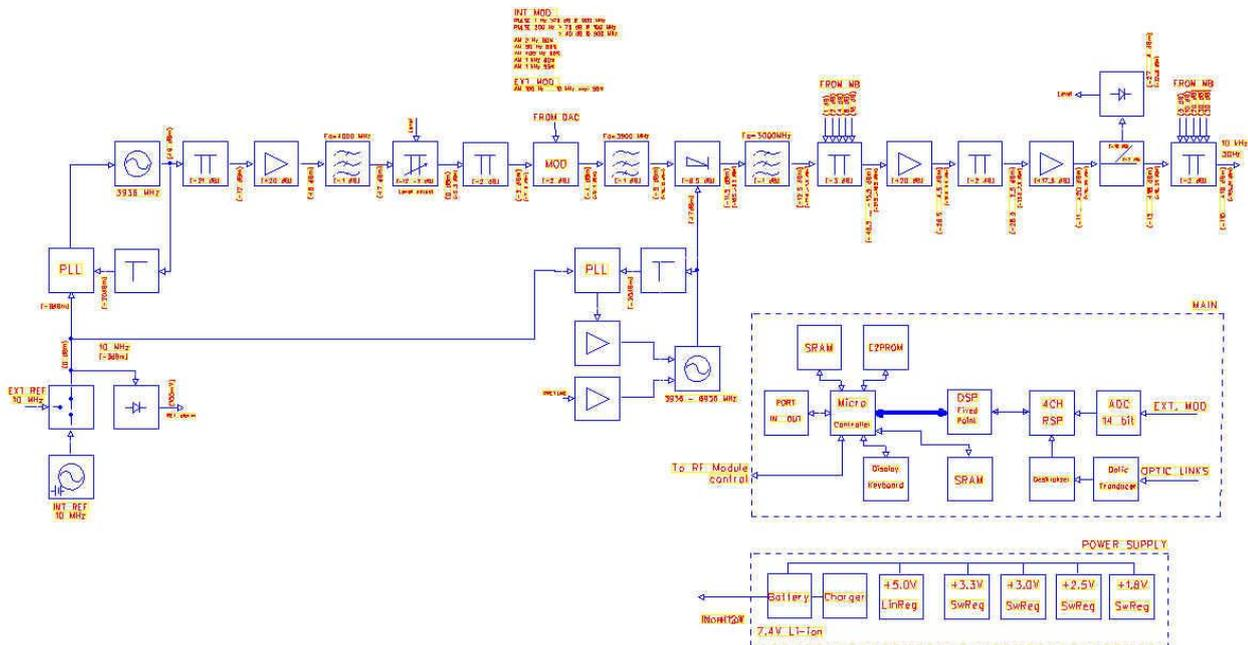
Fig. 1-6 PMM 3010-3030 Functional BLOCK Diagram
